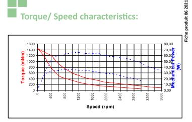
The above statements are given for a 100% value of the setpoint torque and for two supply voltage values (24 and 40
